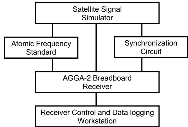
Figure 11: Test hardware set-up
